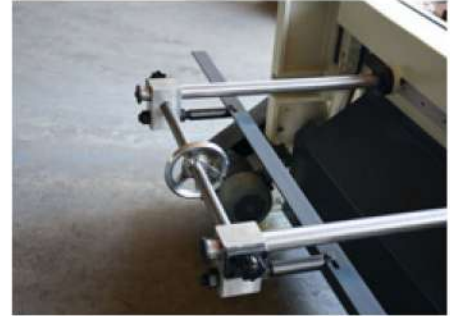
Arka Dayama 600 mm Back Gauge 600mm
